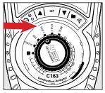
Rotate function rotary dial to FLUE 1 for Flue Test Screen 1 parameters.
