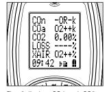
Flue 2 displays CO (ppm), CO2, Losses calculated, Excess air %. Make any adjustments needed for proper Combustion and wait for analyzer to display change in readings. (Repeat as necessary).
