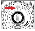
Rotate the function rotary dial to FLUE 2 for Flue Test Screen 2 parameters.
