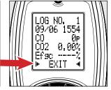
To EXIT. Press ▲ and ▼ buttons until EXIT is selected between two arrow icons. Press to FXIT screen
